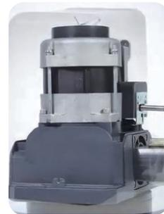
Two options for limits: Mechanical limit and magnetic induction limit
