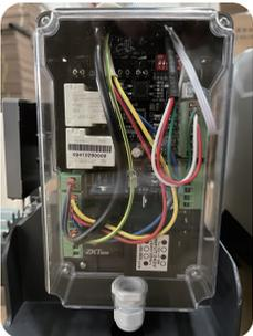
Built-in electronic control waterproof cover, dust and waterproof grade: IP54
